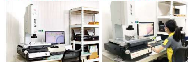
2.5D Projection Measuring Instrument (X-300, Y-200, Z-150)
