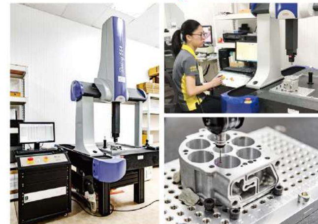
3D Automatic Coordinate Measuring Machine (X-500, Y-600, Z-400)
